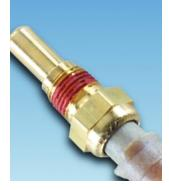
$R_3$  should be set to yield a 0 volt output for 0°C. In both cases, this would be approximately 33K ohms. This can be calibrated with ice water and a thermometer. Care should be taken that the water does not short out the thermistor.
