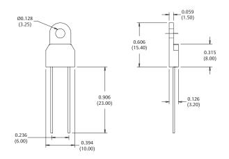
Dimensions are shown in inches and (millimeters).
