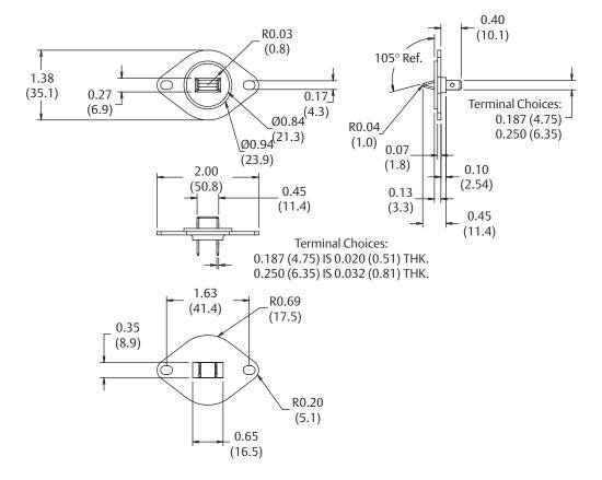
Dimensions are shown in inches and (millimeters).
