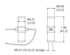
Dimensions are shown in inches and (millimeters).
