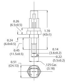
Dimensions are shown in inches and (millimeters).
