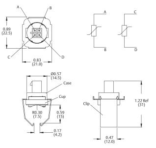
Dimensions are shown in inches and (millimeters).
