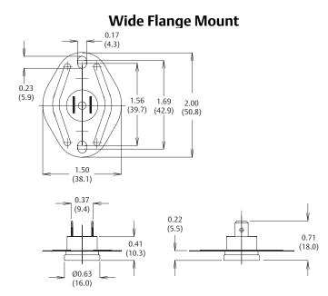
Dimensions are shown in inches and (millimeters).
