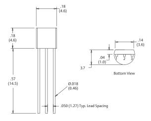
Dimensions are shown in inches and (millimeters).
