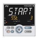
Parameter Setting Display Operation Display > **PARAMETER** key or **PARA** key for **3** seconds (to [MODE] Menu Display) > SET/ENTER key (The setting parameter is displayed.) > Down arrow key (The setting parameter is displayed.)
