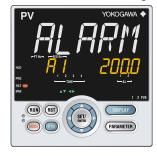
6. Press the SET/ENTER key to register the setpoint (the setpoint stops blinking).
