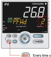
Every time you press the MODE key, the operation mode is switched. Display P.FWD (fast-forwarding), and press the SET/ENTER key.
