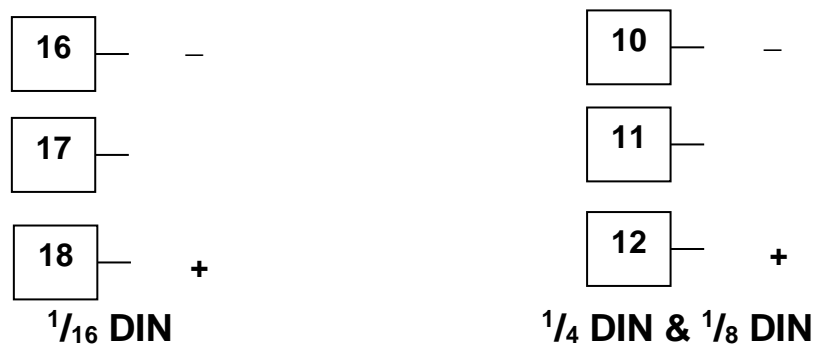
Figure 31. Option Slot 3 - Transmitter Power Supply Module
